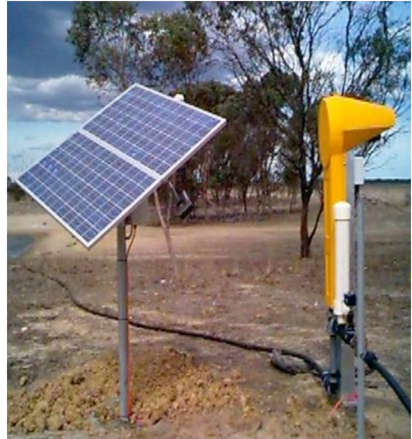
200w "Sunmill" solar pump
