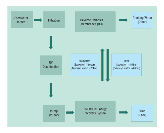
The feedwater flows through filters and an UV-disinfection system to the ENERCON Energy Recovery System. The pump pressure of 20bar is transferred to  $\sim$  56bar/seawater or  $\sim$ 28bar/brackish water and flows to the R0-membranes. At the R0-membranes, feedwater separates into drinking water and brine. Drinking water leaves the system and brine, still under pressure, flows back to the energy recovery system to support the process.
