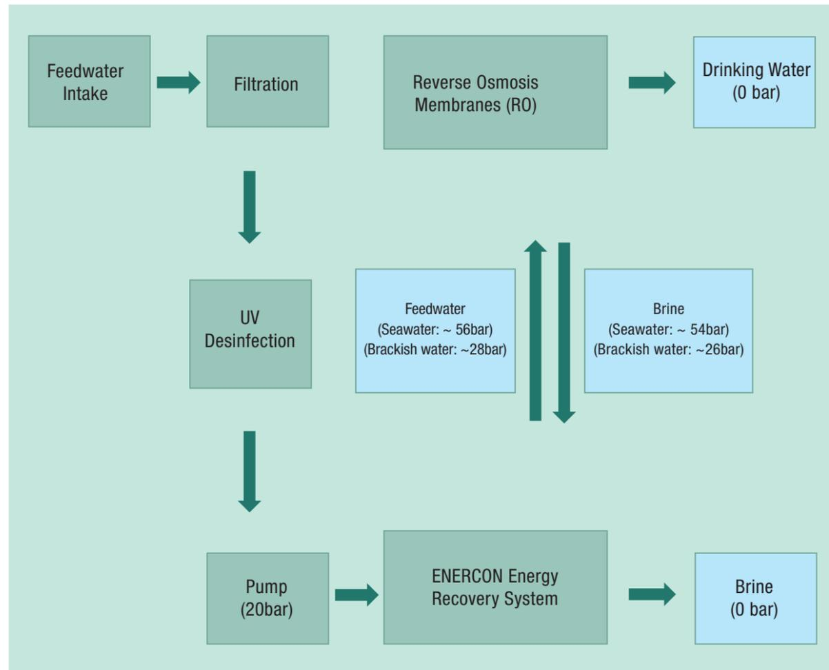
The feedwater flows through filters and an UV-disinfection system to the ENERCON Energy Recovery System. The pump pressure of 20bar is transferred to ~56bar/seawater or ~28bar/brackish water and flows to the RO-membranes. At the RO-membranes, feedwater separates into drinking water and brine. Drinking water leaves the system and brine, still under pressure, flows back to the energy recovery system to support the process.
