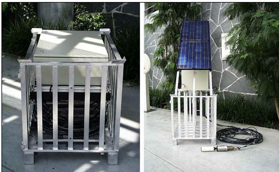
Pic. 40 Water-PPS (pumping and purification system), developed by Fraunhofer ISE
