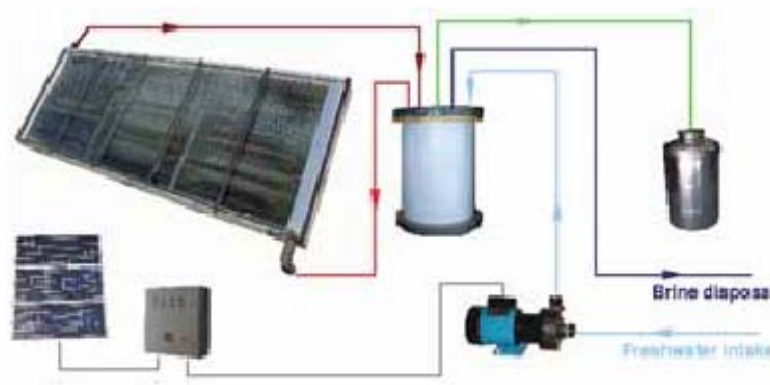
Fig. 42 Sketch of a simple MD-system with production capacity of about 150 l/day.
